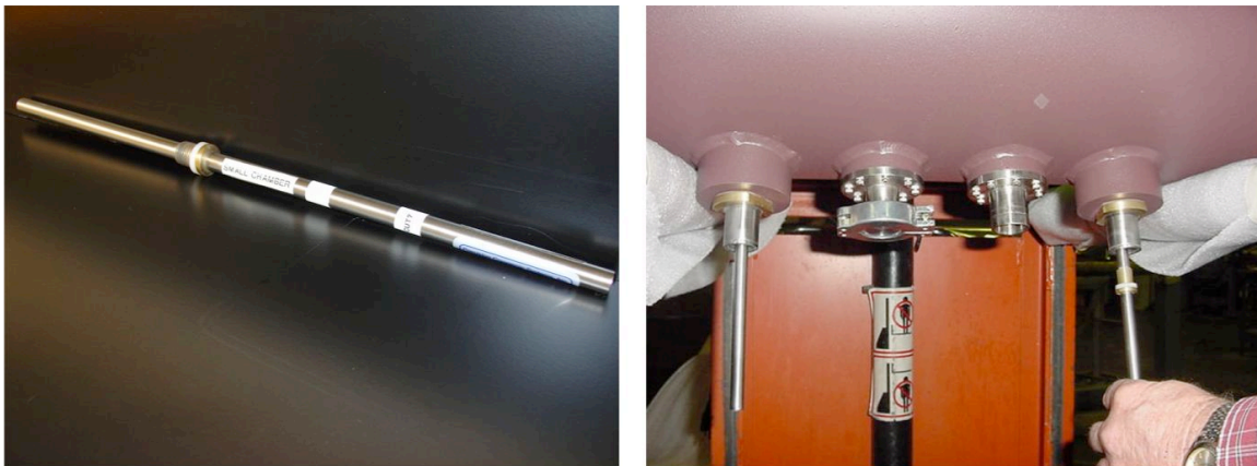
Figure 4. Detail of one of the fill tubes (left), and showing how these are inserted into each tank.
