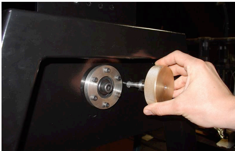
Figure 6. The threaded locking pin on the handling cart. Use care when removing this, as the instrument will immediately rotate when this pin is removed (see photo below).
