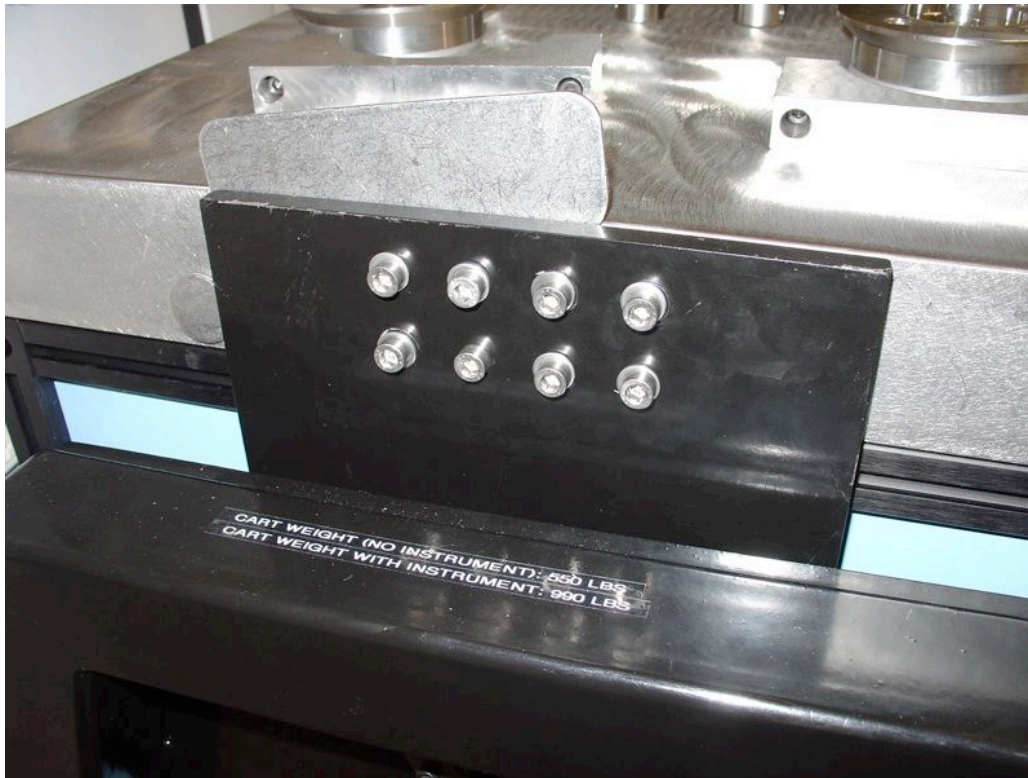
Figure 16. The eight M6 screws used to secure the instrument to each mounting pad on the handling cart.
