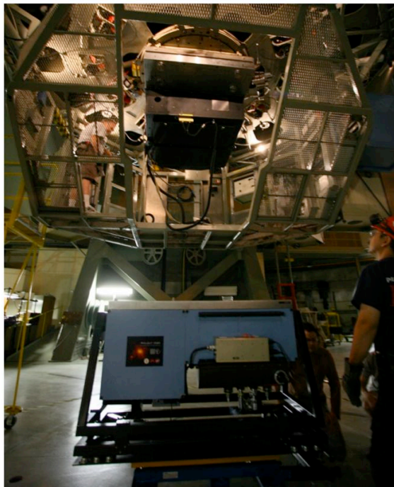
Figure 11. The orientation of the instrument on the Palomar ram must be aligned with its mounting place on the AO system.
