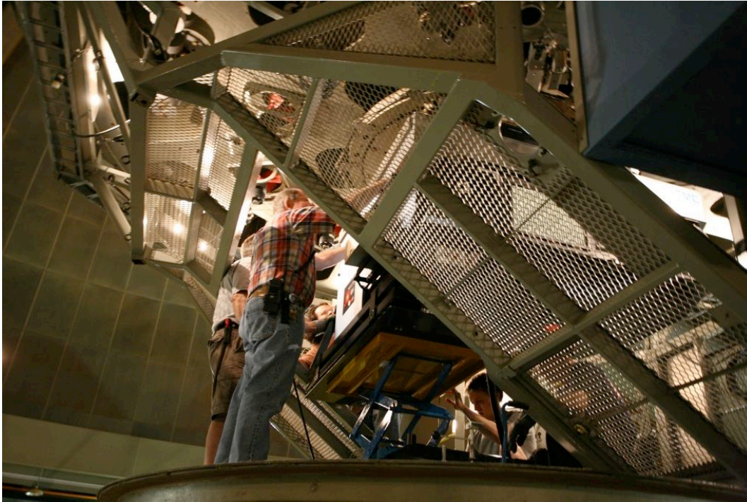
Figure 13. The handling cart should be raised up via its pump mechanism until the yellow portion of the cart platform is higher than the narrowest part of the cage door. Then the cart can then be wheeled towards the middle of the cage.
