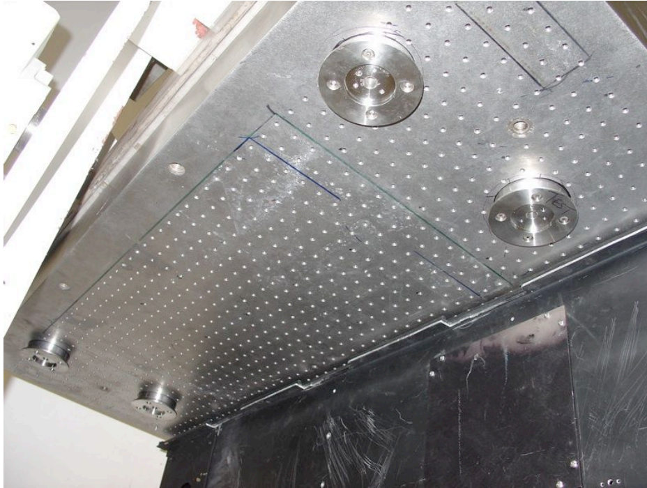
Figure 10. The AO bench showing the four mounting pucks.
