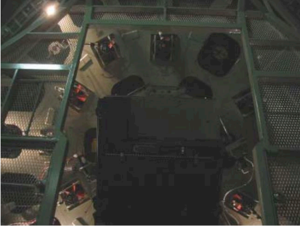
Figure 9. The Cass cage has been rotated into the position needed for mounting.
