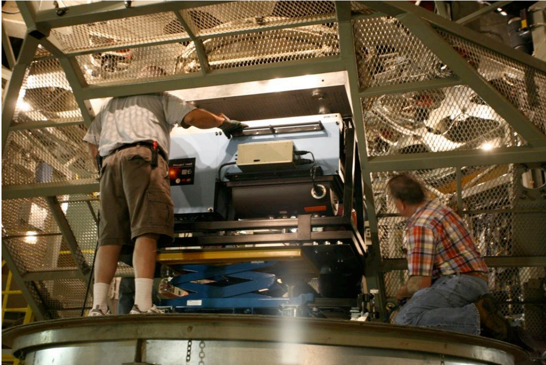
Figure 12. The instrument being raised on the ram through the widest part of the Cass cage door.
