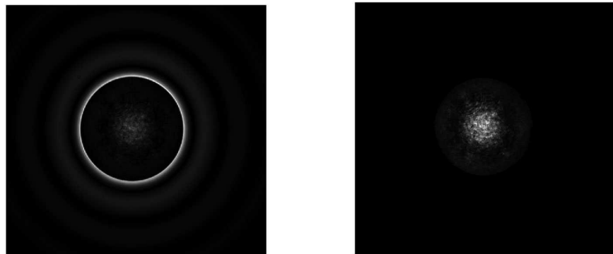
Figure 9. Left: Image of the pupil plane with the apodizer and the FPM in. The light is diffracted outside the pupil. right: Image of the pupil plane with the apodizer, the FPM and the LS in.
