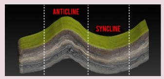
Anticlines and Synclines Tectonic forces can cause rock layers to bend or fold. In an anticline, rock layers are folded upwards in an arch. In a syncline, the rock layers fold downwards.
