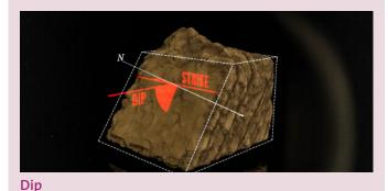
The angle between the fault, or rock layers, and the horizontal surface. Measured between  $0^{\circ}$  to  $90^{\circ}$ .
