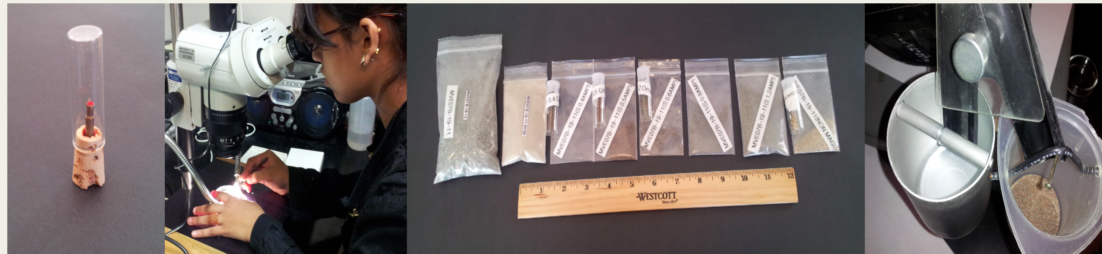
Figure 2. Photo 1: A grain ready for XRD analysis on a fiberglass pin, Photo 2: Samina picking minerals, Photo 3: A fully separated sample, Photo 4: Samples after magnetic separation
