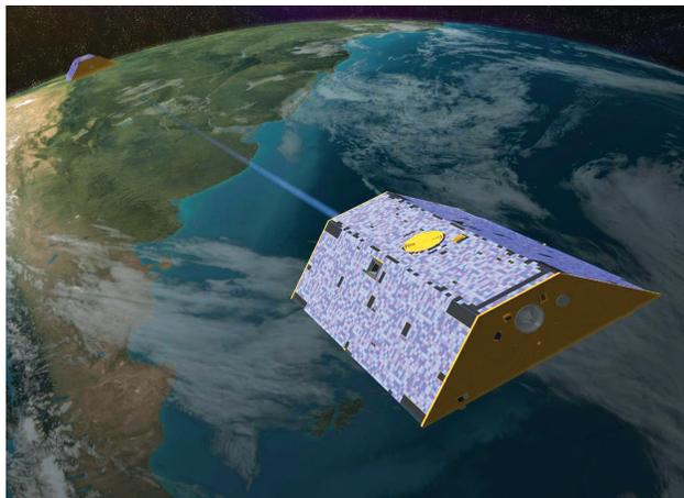
**GRACE, twin satellites launched in March 2002, are making detailed measurements of Earth’s gravitational field.**
