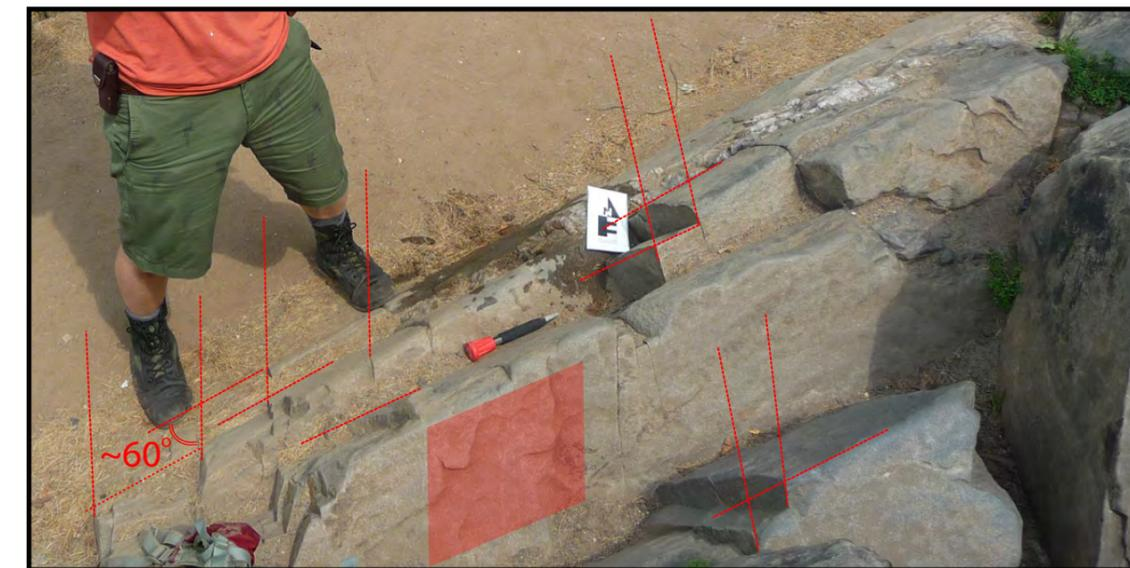
Adjacent image: joint sets observed in the granofels from Hershhead as indicated by dashed lines. Note that one of the three joint sets is in the horizontal plane and is represented by the red rhomboid in the adjacent image.
