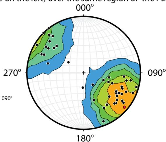
Image below: pole to planes (p plot) from Hershhead with 2s contour interval (larger plot on the right). This plot is excellent agreement with measurements made by Taterka (1987; smaller image on the left) over the same region of the Park
