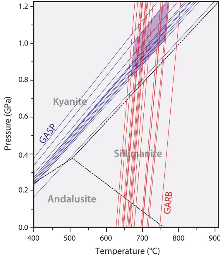
By combining the exchange reaction (red curves; GARB) and the net transfer reaction (blue curves; GASP) at Hershhead we can estimate the P-T conditions at which the rock equilibrated. As shown in the purple shaded region in the adjacent image, the P-T conditions at Hershhead existed at ~1 GPa and ~700 °C. This indicates that the metasediments reached a metamorphic facies of upper amphibolite pressure-temperature conditions.
