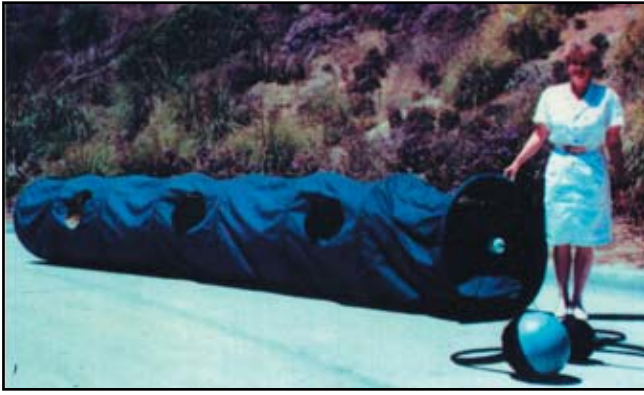
A typical drogue used by oceanographers. This drogue, hanging at a depth of 15 meters and attached to a radio transmitter, ensures that the drifter assemblage tracks shallow ocean currents rather than surface winds. © D. Olson
