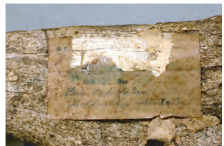
Brittle failure of non-archival paper, adhesive and coating.
