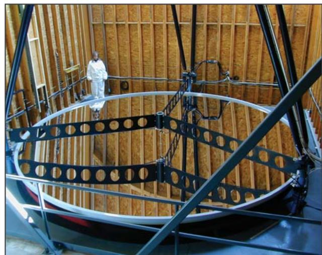
This liquid mirror telescope, the largest on Earth, is 6 meters (20 feet) across. On the Moon, undisturbed by wind or weather, the surface could be larger than a football field.
