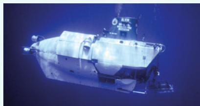
**This submersible takes scientists down 900 meters (3,000 feet). On-board cameras record underwater scenes while a robotic arm and samplers collect specimens.**
