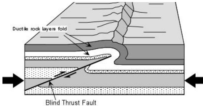
This illustration shows how a blind thrust fault can form an anticline. The large arrows indicate the direction that force is being applied. Image courtesy of Stephen Nelson, Tulane University
