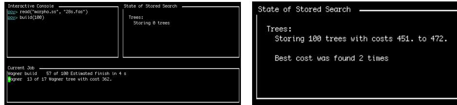
Figure 2.23: Generating Wagner trees. During the process of tree building (left panel), the Current Job window displays how many builds have been performed so far (57 of 100), the number of terminals added in the current build (13 of 17), the cost of a current tree recalculated after each terminal addition (362), and the estimated time (in seconds) for the completion of the operation (4 s). Because the process is not complete, the State of Stored Search window contains no trees. Once tree building is complete, the State of Stored Search window displays the best (451) and worst (472) costs, the number of trees stored in memory (100), and the number of trees with the best cost (2).
