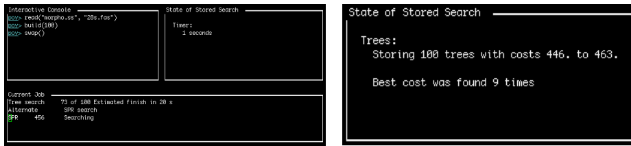
Figure 2.24: Performing a local search. When searching (left panel), the Current Job window reports the number of the tree that is currently being analyzed (73 of 100), a method of branch swapping ( Alternate ), a function being currently performed ( SPR search ), and a cost of the current tree (456). When the searching is finished (right panel), the State of Stored Search window displays the best (446) and worst (463) costs, the number of trees stored in memory (100), and the number of trees of the best cost (9) recovered from independent tree builds and swaps. Notice that these trees may not necessarily have unique topologies.
