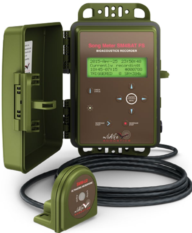
Figure 4. The SM4Bat recorder and microphone made by Wildlife Acoustics. The recorder can be programmed to record at specific times. Bat researchers typically record from 30 minutes before sunset to 30 minutes after sunrise, when most bat species will forage for food.
