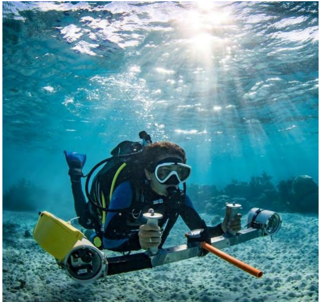
Figure 2. SCUBA diver conducting diver operated video (stereo-DOV) survey at Mo'orea, French Polynesia. Photo credit: Lauric Thiault/Goetze et al. 2019.
